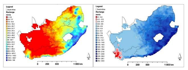
Figure 3-3 Recharge distribution maps of South Africa displaying current recharge conditions (left) and the change in annual recharge between the current and future (right) by Dennis et.al (2012).
